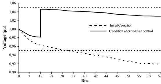
Figure 4 -Voltage profiles of main feeder to peak load condition.
